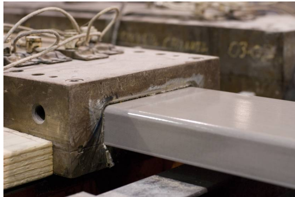
Heated die cures resin
