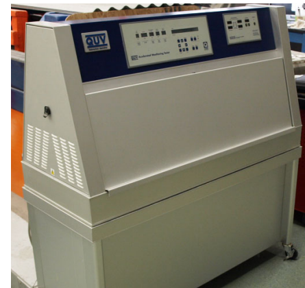
QUV (ultraviolet/ accelerated weathering)
